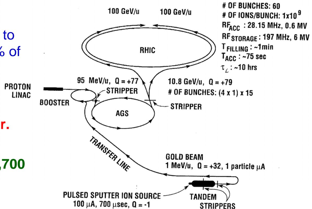
Fig. 2. RHIC acceleration scenario for Au beams.
