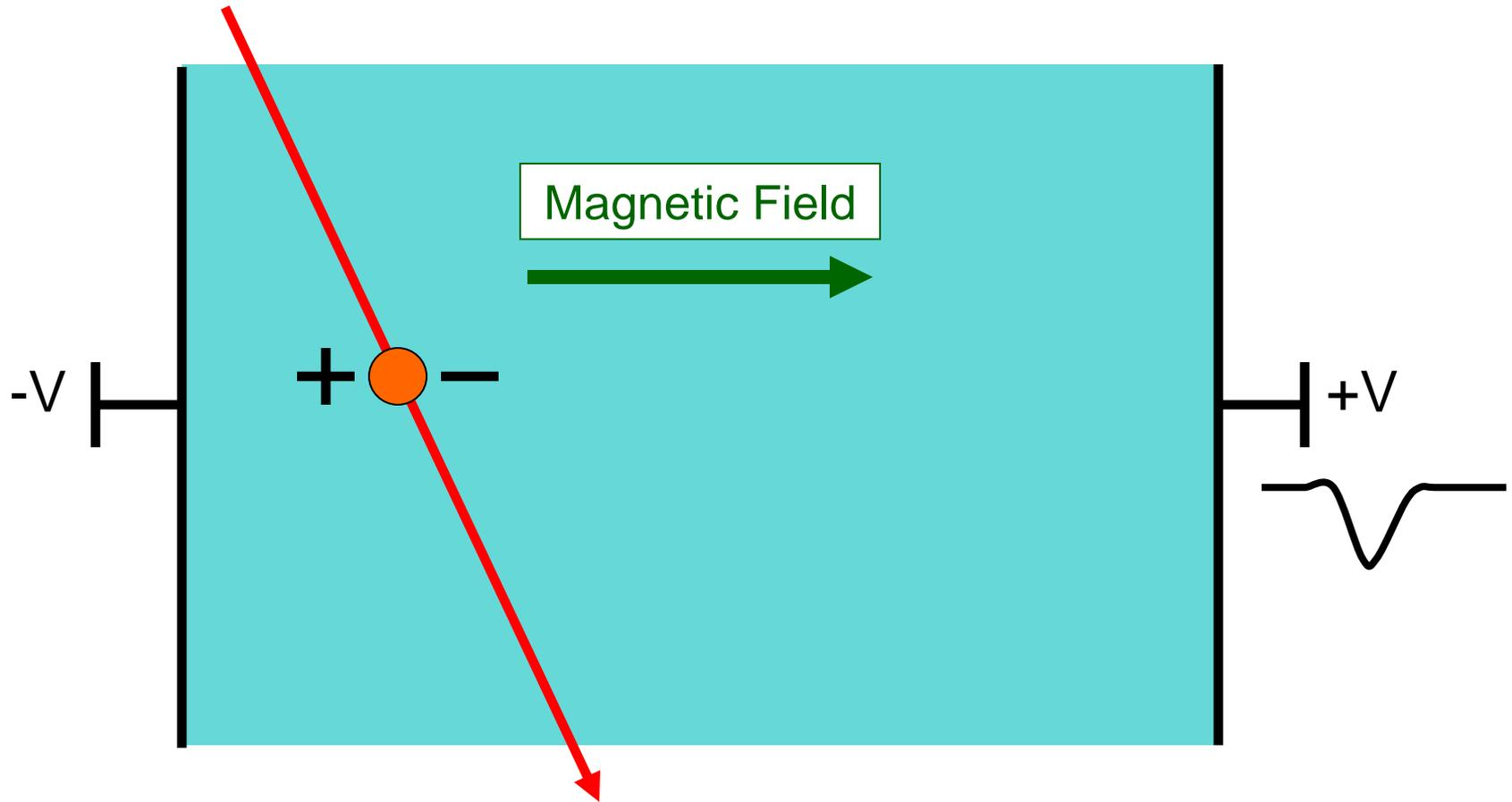
The time to reach the end of the TPC determines the distance drifted in the gas.
